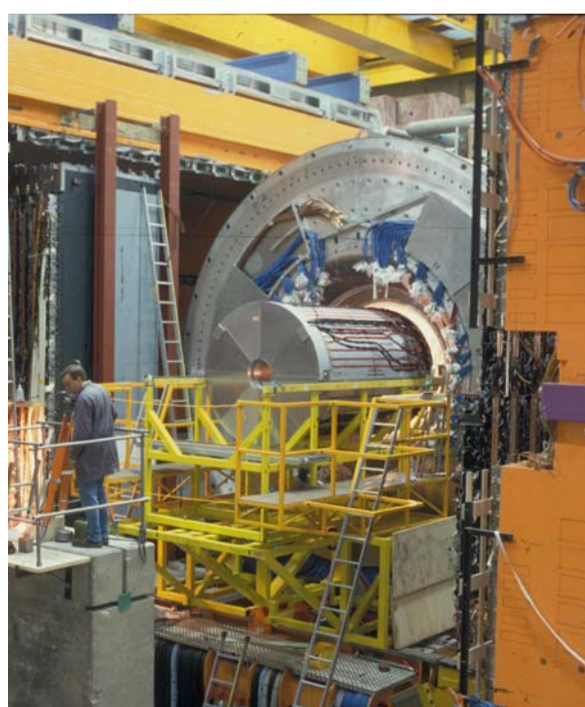
Installation of the CTD in the ZEUS hall
